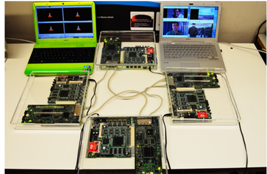
Figure 2: Demo network with ARP-Path 4*1 Gbps switches
