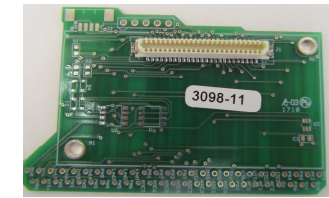
Fig. 3: Interface board to connect IRIS mote and iRobot
