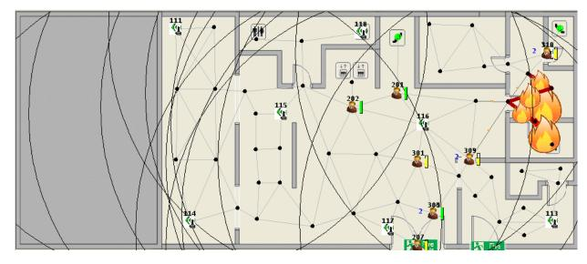
Fig. 1. Sample screen capture of the Building evacuation simulator
