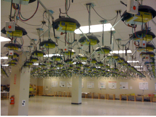
Fig. 2. The ORBIT testbed with 400 WiFi enabled nodes arranged in a grid topology.
